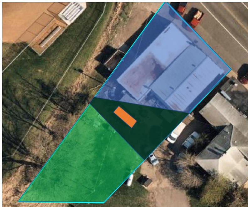
Figure 3 100' Setback from County Roads Applied to Property
