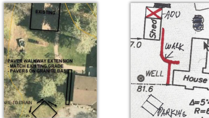
Figure 8 Grading & Site Plan Showing Walkway
